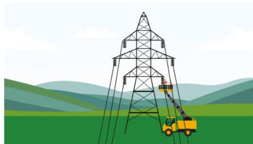
Stage 4: Attaching the wires
