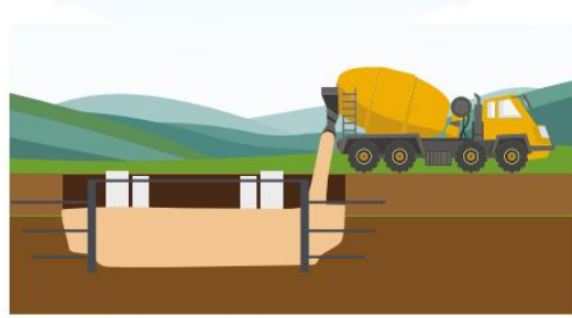
Stage 2: Pylon foundations
